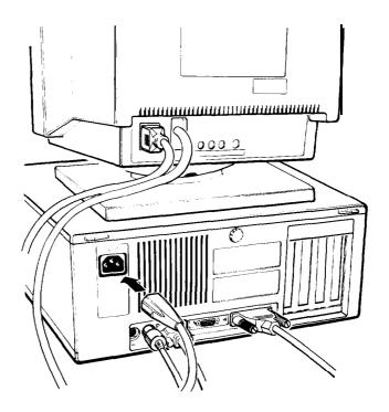
2. Plug the other end of the power cord into a three-hole, 120-volt, grounded electrical outlet.
